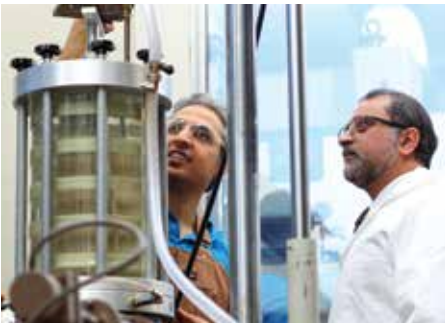
ABOVE: HANY EL NAGGAR AND MOHAMMAD ASHARI CARRYING OUT LARGE-SCALE TRIAXIAL TESTING OF TDA/SAND MIXTURES.
