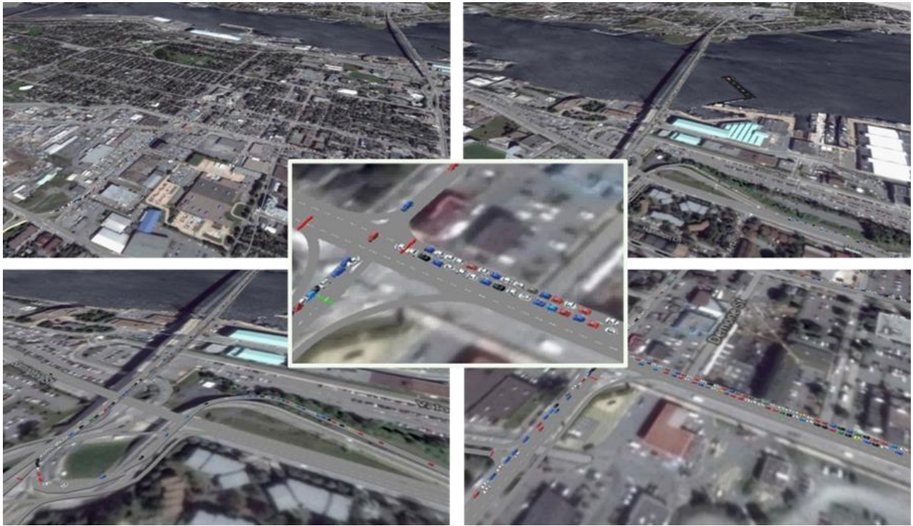
Figure: Visualization of the traffic evacuation microsimulation model, traffic evacuation and congestion in the Halifax transport network
