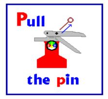
**PULL** the pin at the top of the extinguisher
