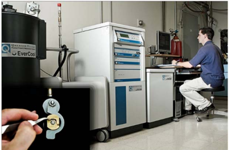
Figure 21. (a) Lab-built adiabatic calorimeter that I built at the University of Waterloo and brought with me to Dalhousie in 1983. (b) The PPMS with Mike Johnson running the instrument, and an inset of the heat capacity platform.
