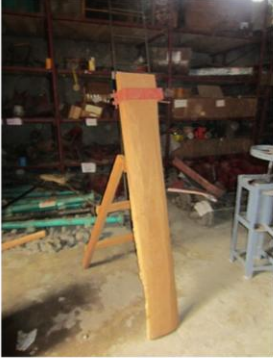
Enset Scapper with metal clip to improve sanitation during processing. Contrary to reports from technology developers and researchers, the women in this research did not use their feet to hold the sheath to the scrapper. They used rope to hold the sheath to the board.
