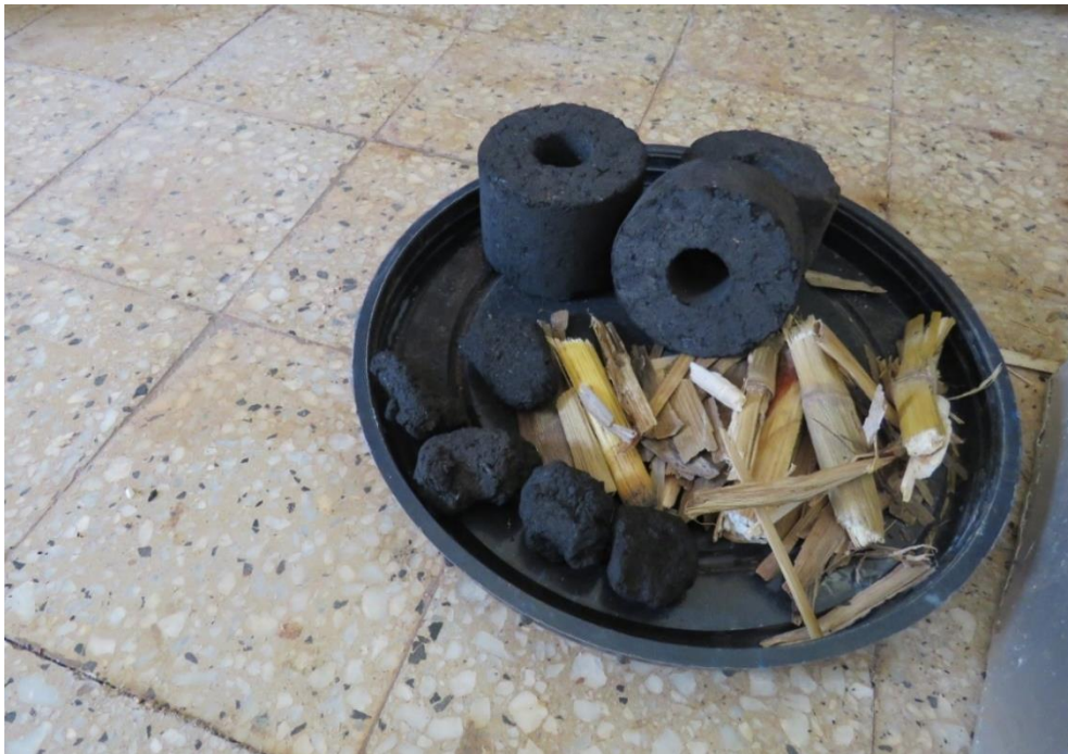
Figure 4: Charcoal briquettes produced at Wolaita Soddo ATVET alongside the raw materials
