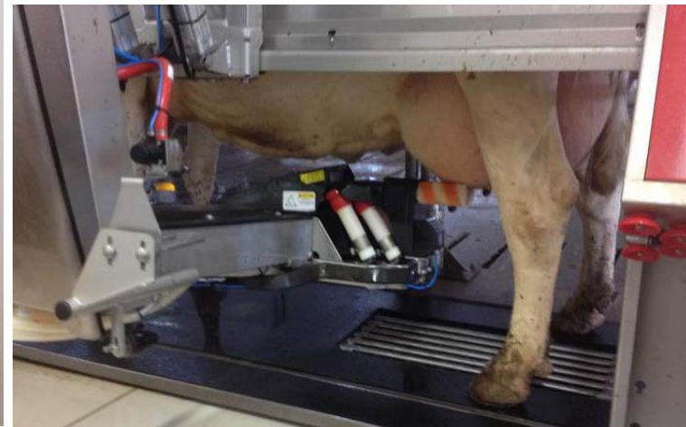
The milking robots used at Vissers Farm near Stewiacke, similar to ones that have been used in the auto industry for years, identify each cow via a transponder, determine when she was last milked and her position in the stall, and then gently hook her up to a vacuum milker. CONTRIBUTED
