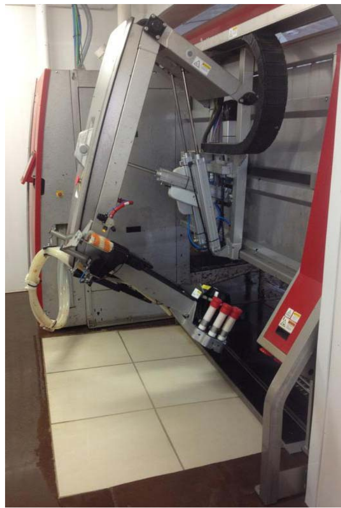
The milking robots used at Vissers Farm near Stewiacke, similar to ones that have been used in the auto industry for years, identify each cow via a transponder, determine when she was last milked and her position in the stall, and then gently hook her up to a vacuum milker. CONTRIBUTED
