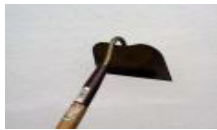
Note the beveled edge of the draw hoe. The angle of the blade allows a chopping action before each draw of the hoe. © Sherry Chaisson & Stuart Gibb, Dalhousie.
