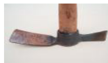
The axe-mattock allows you to dig in root-filled soil. The broad blade moves and loosens soil while the axe cuts through roots. © Sherry Chaisson & Stuart Gibb, Dalhousie.
