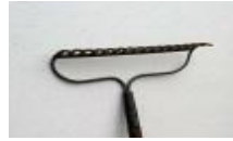
The bow rake allows stones to pass through the opening. It is used for deep raking. © Sherry Chaisson & Stuart Gibb, Dalhousie.
