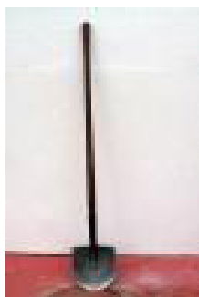
This round-nosed shovel is ideal for moving soil. The long handle allows for good leverage. © Sherry Chaisson & Stuart Gibb, Dalhousie.
