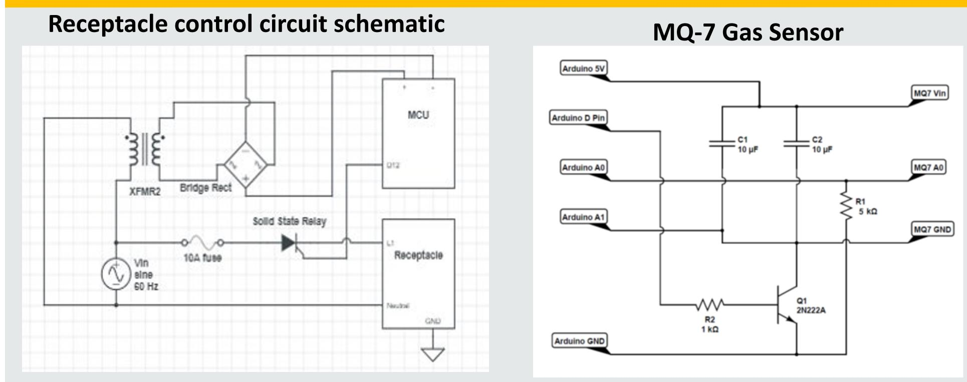
Once a CO PPM of 20 or greater has been detected, the MCU energizes the SSR relay, which supplies the receptacle with power, allowing user added devices to alert or remove the gas.
