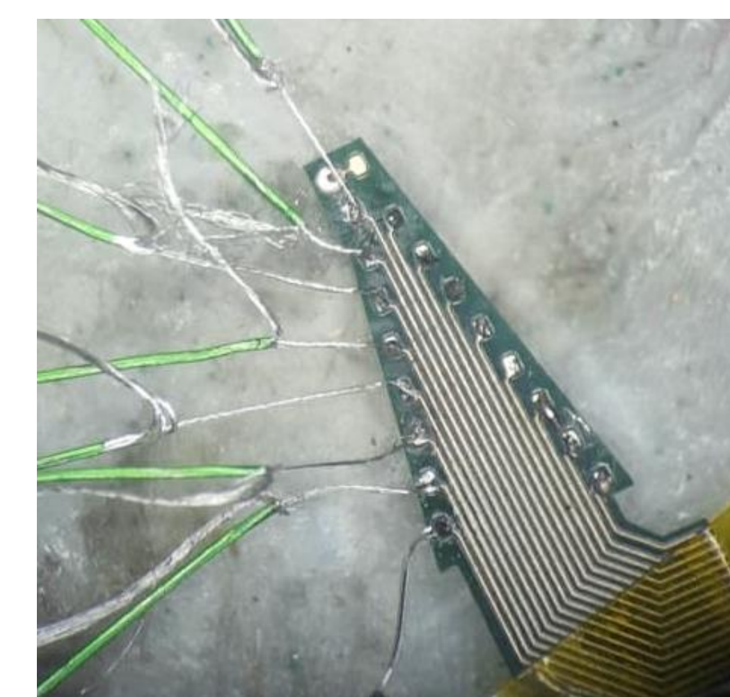
Figure 5: Cables Soldered to PCB
