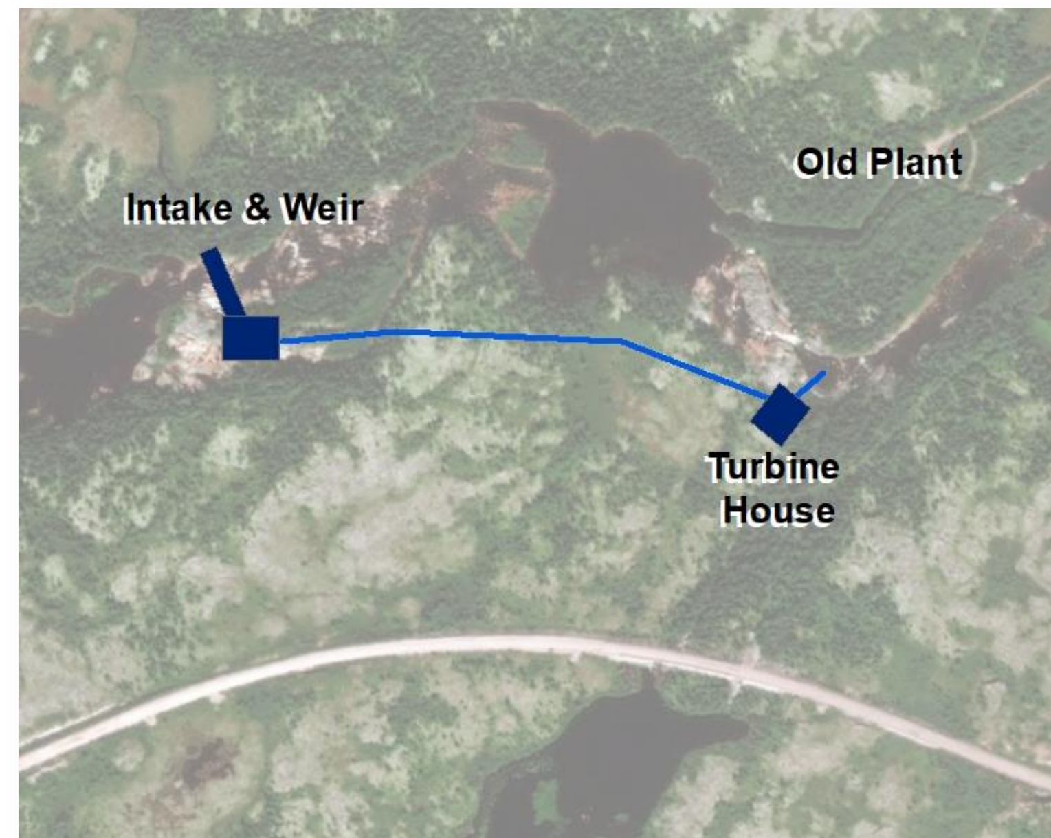
Figure 3 Proposed Penstock to Turbine layout
