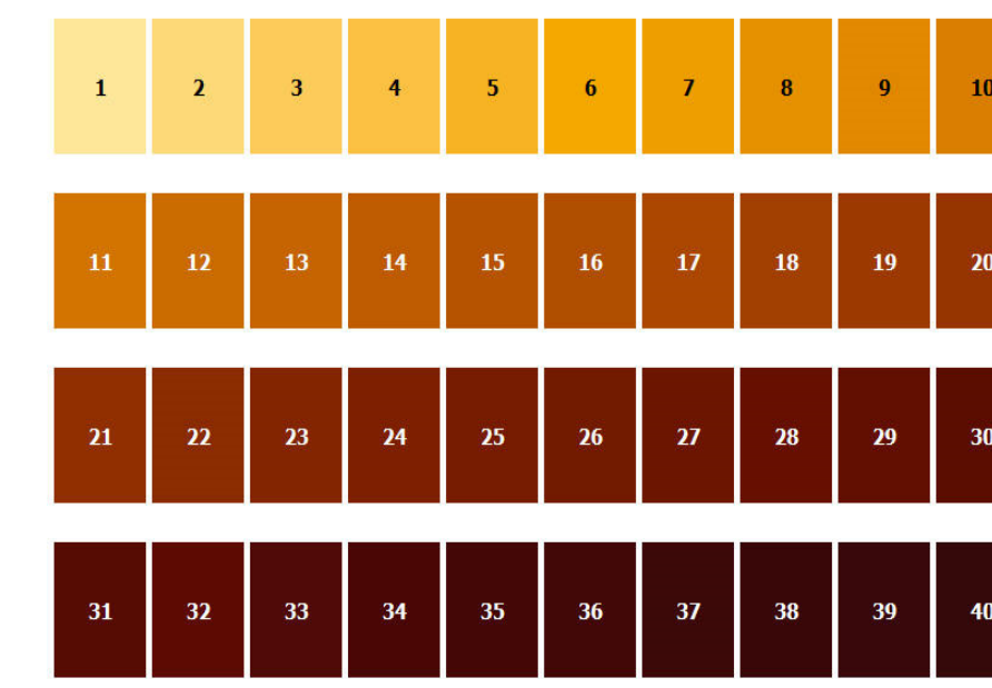
Figure 4: Gardner color scale (ASTM-D1544).
